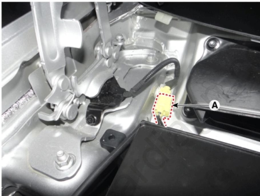
4. Remove the active hood actuator by loosening the bolt (A).
